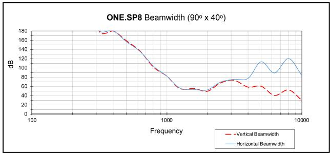
NOTE: These measurements were created using EASE software, which limits the bandwidth to 100 - 10,000 Hz that is critical for full-range loudspeakers. No processing was used.
