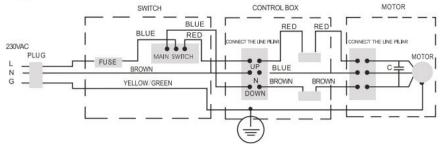
If the motorized screen work with remote control, please refer to the below fig for electric connection.  $_{\text{CONTROLBOX}}$   $_{\text{MOTOR}}$
