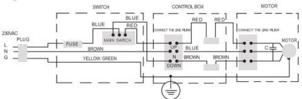
If the motorized screen work with remote control, please refer to the below fig for electric connection.
