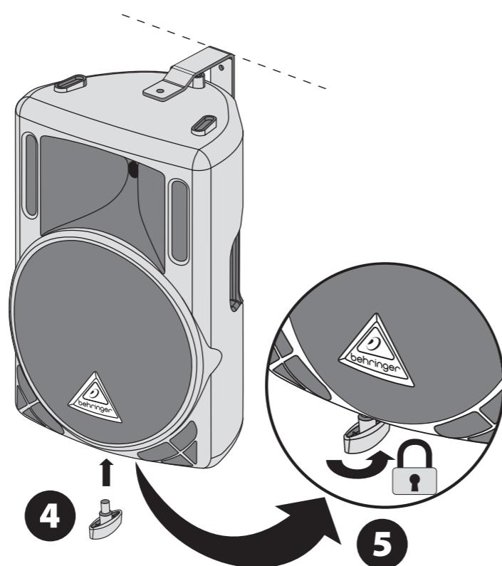
**4** **[EN]** Insert the MOUNTING POLE FASTENER into the MOUNTING POLE from below through the hole in the lower bracket.
