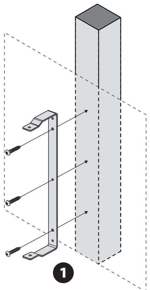
**1** **[EN]** Secure the mounting bracket to the wall by running screws through the MOUNTING SCREW EYELETS (vertical mounting only; screws and other fasteners not included).
